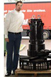
Product expert Carsten Bode: TRN submerged aerators work along the same principle as submersible pumps, however they move air, not water. This means they are practically fail proof even if used permanently. (Photo: Tsurumi)
