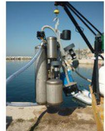
The project presents a number of technical challenges. Getting to the sludge itself is among the hardest as this can only be attempted through existing openings on the top of each vessel, and these measure just one metre across. To cope with the size restrictions and yet ensure that every corner of the silo is reached, a novel idea was conceived: a Tsurumi pump connected to a ROV will travel around the silo pumping sludge to a downstream treatment unit.
