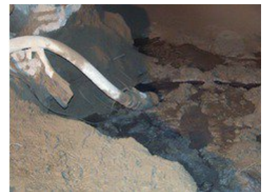
Sediment gives no pumping problems "Silt Pumping: Large particles of sediment in the medium pose no problems for cascade-connected pumps"
