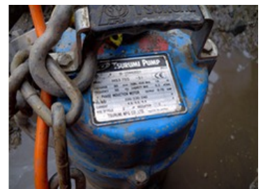
A quick glance at the name plate: Is all the information provided and plausible? (photo: Tsurumi)
