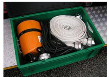
A Tsurumi LSC puddle-sucking pump with hose in a compact and transportable box
