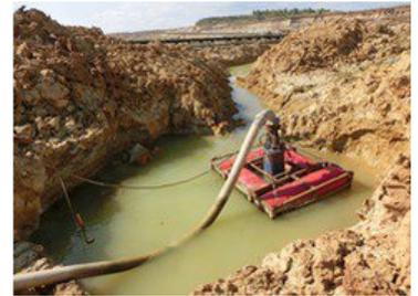
Tsurumi pump in its element: Just 16 pumps keep the Visonta mine with its 4.8 million tons of annual production dry (Photo: Tsurumi)
