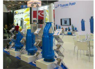
Tsurumi presented several innovations including the KRSU822 (shown at the front in the photo) as a pump with a 56 mm clear passage for heavy media (photo: Tsurumi)
