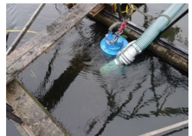
The submersible pump hangs on a chain, meaning it can be freely positioned (photo: Tsurumi) Download photo
