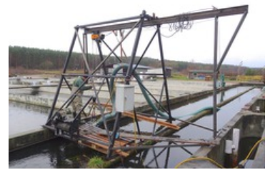
Pump instead of excavator: The channel with pump at the front and the tank where the sludgy problem comes from behind. The channel had to be dredged once a year up until now (photo: Tsurumi) Download photo
