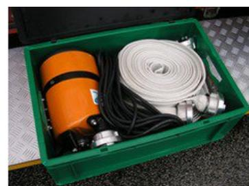
A Tsurumi LSC puddle-sucking pump with hose in a compact and transportable box
