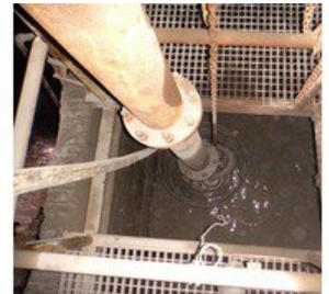
Pump sump with a riser: more than 100 pumps from Tsurumi are used to pump water in the mine (Photo: Tsurumi)
