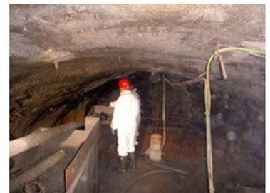
Pipelines gradually pump groundwater from the head of the mine up to the surface (Photo: Tsurumi)
